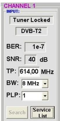
The quality of the input signal can be evaluated using the bit error ratio **BER** and the signal-to-noise ratio **SNR**.
