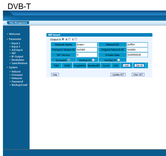
Pic. 17: Creating a NIT and assigning LCN using the example of the HDS 4 T01
